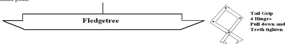
On the hoist wire to the fledgetree, was a tail grip contraption. This would grip the tail tip and tighten on the tail as any pressure was applied to the tail hide.
