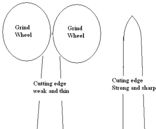
*His explanation was to think of the knife steel blade as a wedge of cheese, if you grind the wedge with a hollow each side of the sharp edge the sharp edge will crumble and never stay sharp for long.*
